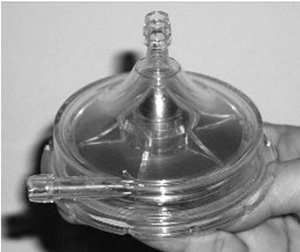
Figure 9.6 A typical centrifugal pump head, the pump head is shown separated from the drive mechanism. The impeller can be seen in the pump head and the drive magnets are apparent at the base of the mechanism.
