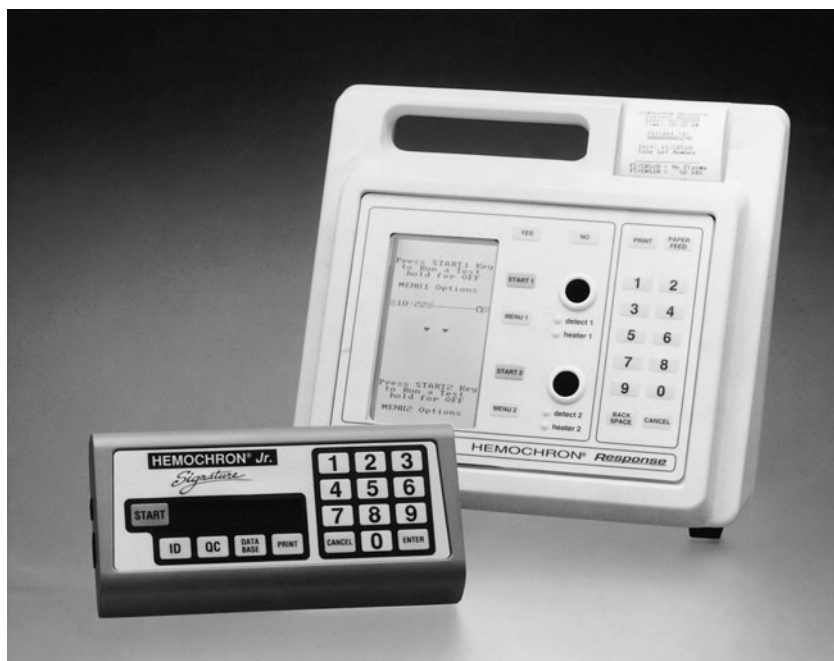
Figure 13.6 The Haemochron Response and the Haemochron Jr. ACT device (International Technidyne Corporation L) used for monitoring anticoagulation during cardiac surgery.
