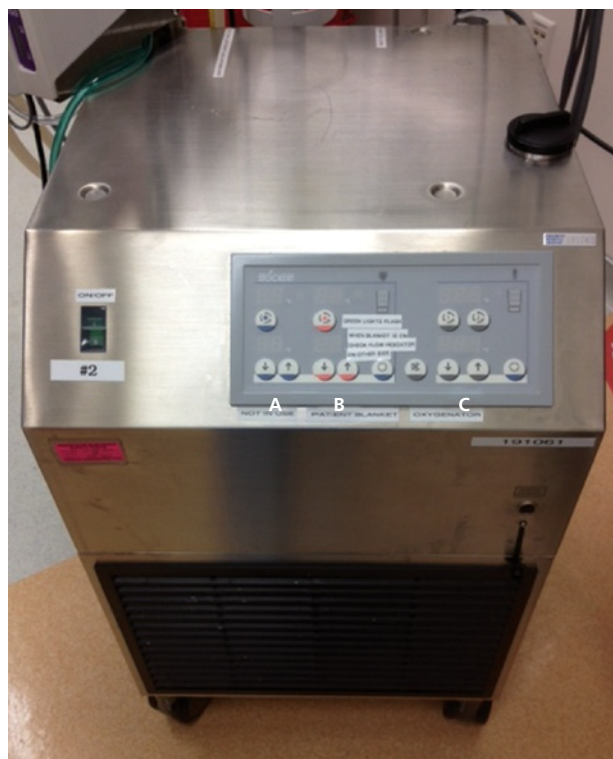
Figure 1.14 Stockert heater-cooler system 3T (three-tank system). A—Cold cardioplegia circuit. The first tank instantly provides 2–10°C water to the cardioplegia system. B—Warm cardioplegia circuit. The second tank instantly provides 15–41°C water to the cardioplegia system. It can also be fitted for a water-based patient surface cooling/heating blanket. C—Oxygenator circuit. The third tank provides 15–41°C water to the oxygenator heat exchanger. It has a second pump and circuit to provide water flow from the same tank to a water-based patient blanket if desired. (See insert for color representation of the figure.)
