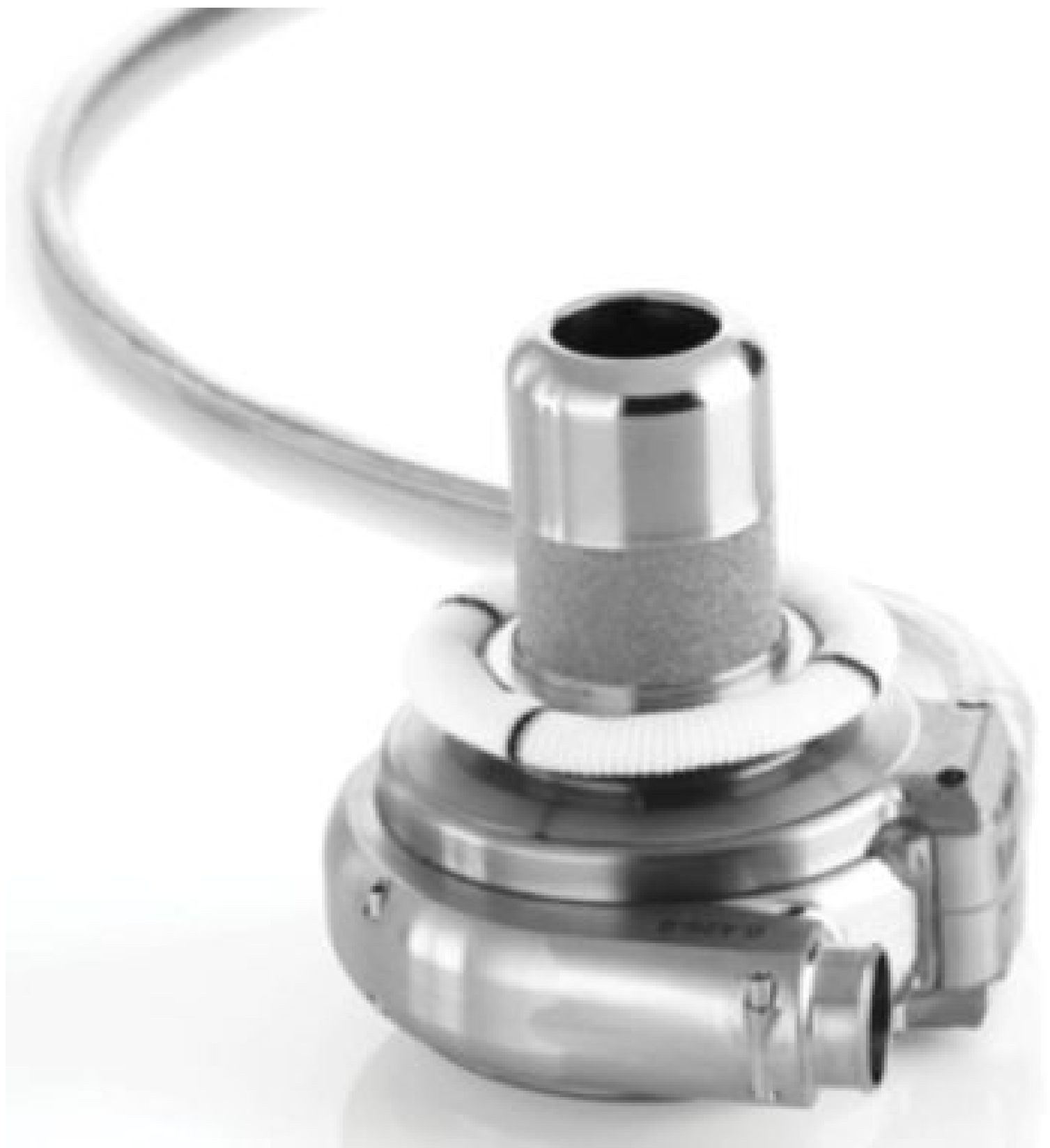
Figure 9.9 HeartWare HVAD pump integrated sintered inflow cannula, driveline, and sewing ring used to attach the pump to the left ventricle.
