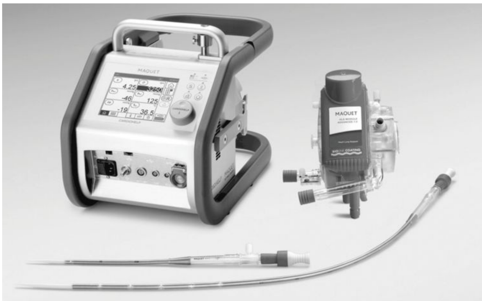
Figure 16.1 CARDIOHELP System is one of the first fully portable emergency life support systems for patients suffering cardiogenic shock. It measures 31 × 25 × 42 cm and weighs 11.5 kg with an ability to generate up to 6 l/minute flow with peripheral or central arteriovenous cannulation.
